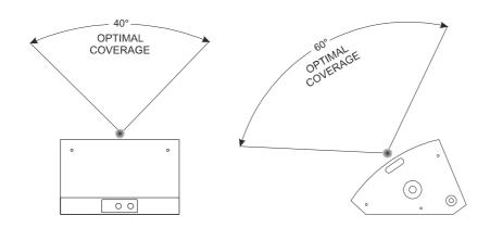
Loudspeaker's horn is rotable of 90°, this allow to invert the optimal coverage areas. To rotate the horn, use an M4 hex key, remove the screw in the inner side, rotate the external of the horn, then tighten the screw.
