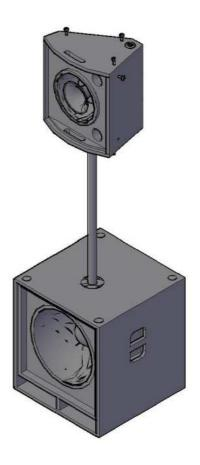
For suspended installation, there are six brackets inside the case: three in the left side, three in the right side. Each bracket is secured to two adjacent internal side of speaker using two M10 screwbolts.
