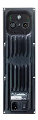
Before making connection between mixer and active speaker, make sure all the switches of the speakers are turned off and the mixer volume is turned down. To avoid a sudden signal, making connection, then turn on the mixer first and then the speakers. Turn on the amplifier by the power switch to position 1 (on).
