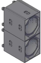
It is possible to install more OCTO21A in stack configuration making fit Top Sub's plastic skids in bottom sub's recesses.
