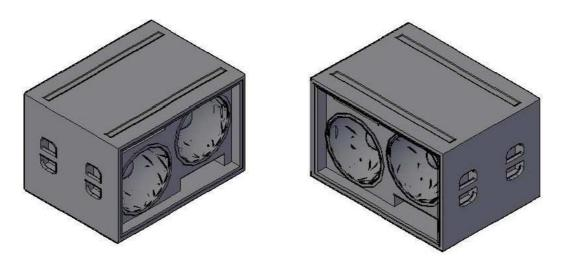
It is possible to install more PSUB2 in stack configuration making fit Top Sub's feet in bottom sub's recesses
