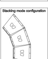
QREX can be installed stand-alone or in multiple configuration. Multiple installation of QREX can be done both in stack or fly configuration. Each loudspeaker has a fixing system that allows to be connected and secured to the other loudspeaker.
