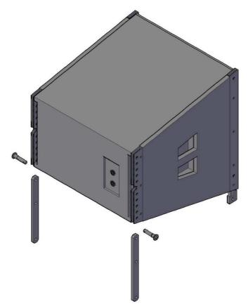
When more QREX are installed in stack, they must be locked using the clamping brackets. Maximum 3 QREX can be installed in stack or fly configuration. The first QREX have to be placed on the BUMPERQREX support. BUMPERQREX increases stability in stack configuration.
