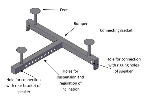
In case of installation in Stacking mode, install the feet and mount the speakers.
