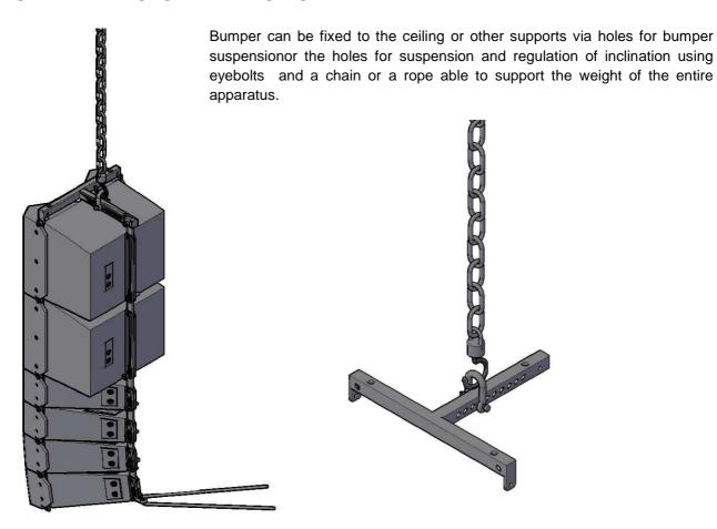
Suspending the bumper from holes for suspension and regulation of inclination, it is possible to determine the inclination of the entire system. Inclination value depends from hole and speakers used because of varying the number of speakers, change the center of gravity, so for an exact operation use an inclinometer.
