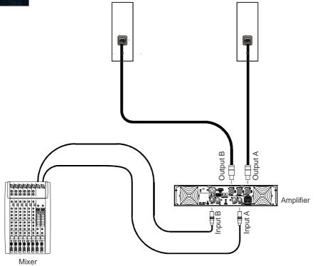
Recommended configuration using multiple speakers is represented below:
