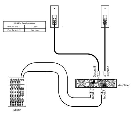
00 000 Output A Output B Ģ Amplifier Amplifier Load (per Output Channel) Nominal Minimum # of Speakers Input B 7 Ohms 8 Ohms 1 2 4 Ohms 3.5 Ohms Input A 2.7 Ohms 2.3 Ohms 3 4 2 Ohms 1.8 Ohms NL4 Pin Configuration Caution: Do not exceed the Pins 1+ and 1-Used maximum load rating of the amplifier. Pins 2+ and 2-Not Used Mixer
