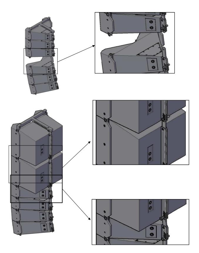
The regulation holes of the bracket allow to choose the desired inclination of the top speaker than the bottom speaker.
