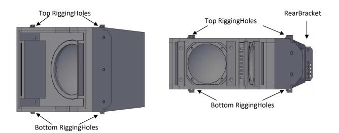
The bracket with rigging holes has a female side and a male side in order to facilitate the snap-in mounting of more speakers.
