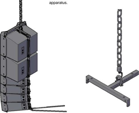
Suspending the bumper from holes for suspension and regulation of inclination, it is possible to determine the inclination of the entire system. Inclination value depends from hole and speakers used because of varying the number of speakers, change the center of gravity, so for an exact operation use an inclinometer.
