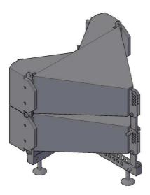
In case of installation in Flying mode, use the bumper without feet, attach the speaker to the sides via rigging holes, then connect the rear bracket adjusting the inclination.
