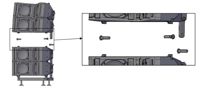
Overlap the speakers aligning the rigging holes, then secure them with the quick release pins.
