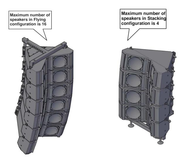
It is recommended touse ST17 together with the sub SB17. They have the same mounting hardware and similar shape in order to facilitate the creation of arrays.
