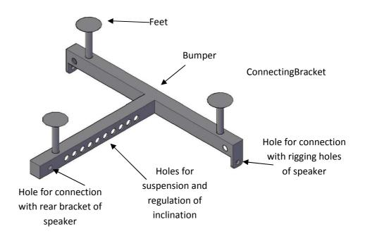
In case of installation in Stacking mode, install the feet then mount the speakers.
