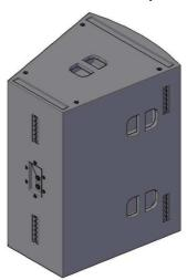
In the bottom of the case there are two plastic skeeds used as feet to support the sub.
