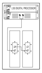
TREX system operating mode is only Bi-Amp (LF 1- 1+; HF 2- 2+) and needs an external digital processor with custom setup provided by LSS. on request it is possible to ask setting parameter in order to use third part processor. If your amplifier can manage a 2 Ohms Load and has sufficient power, it is possible to connect a maximum of 4 speaker in parallel (total impedance will be 2 Ohms).
