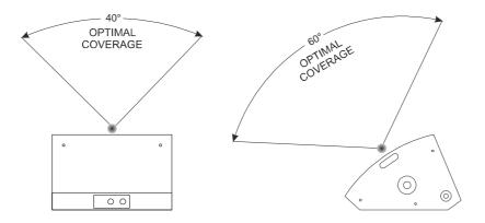
Loudspeaker's horn is rotable of 90°, this allow to invert the optimal coverage areas. To rotate the horn, use an M4 hex key, remove the screw in the inner side, rotate the external of the horn, then tighten the screw.
